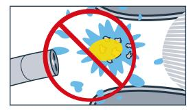
Attention: If component K2 is injected too quickly, component K1 may be washed away.
